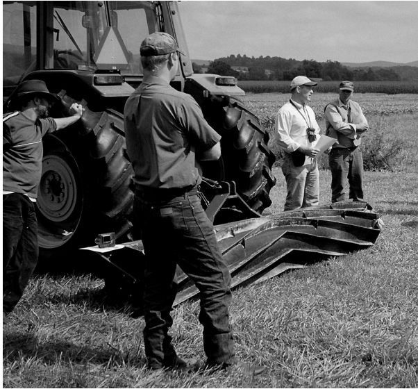
Figure 2. The roller-crimper (left) has been developed specifically for no-till management of high biomass cover crops. The flail mower (right) is a versatile tool, in that it can be used to generate even, finely chopped mulch, or can be operated with the PTO off to function as a roller, as shown here.
