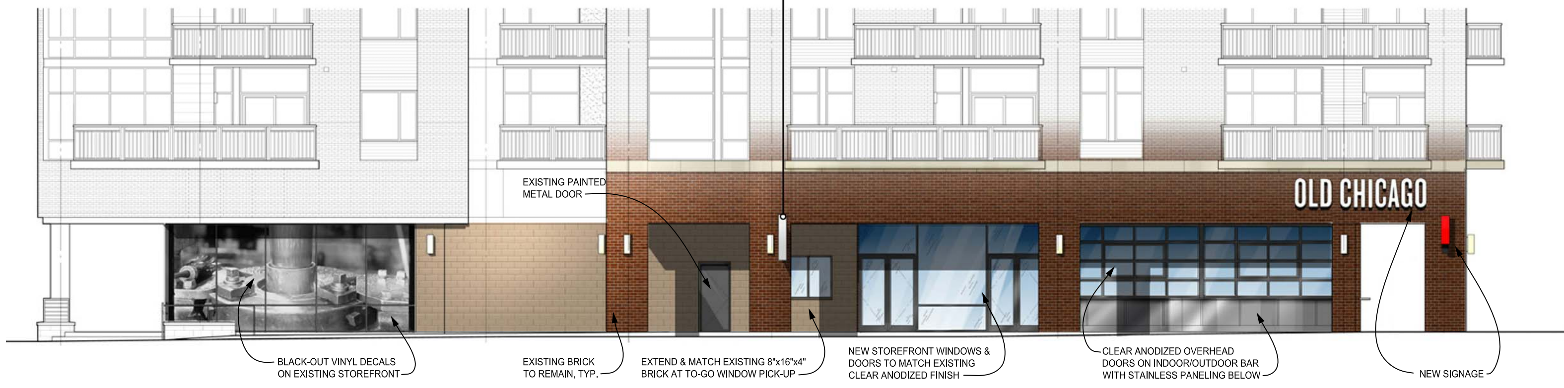
1 WEST ELEVATION (CHURCH STREET) A3.1 1" = 10'
